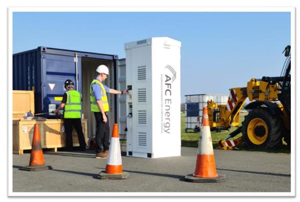
10kW Power Tower EV with integrated Type-2 AC Charger
