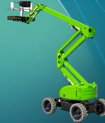
Battery / H 2 Powered Access 1kW FC
